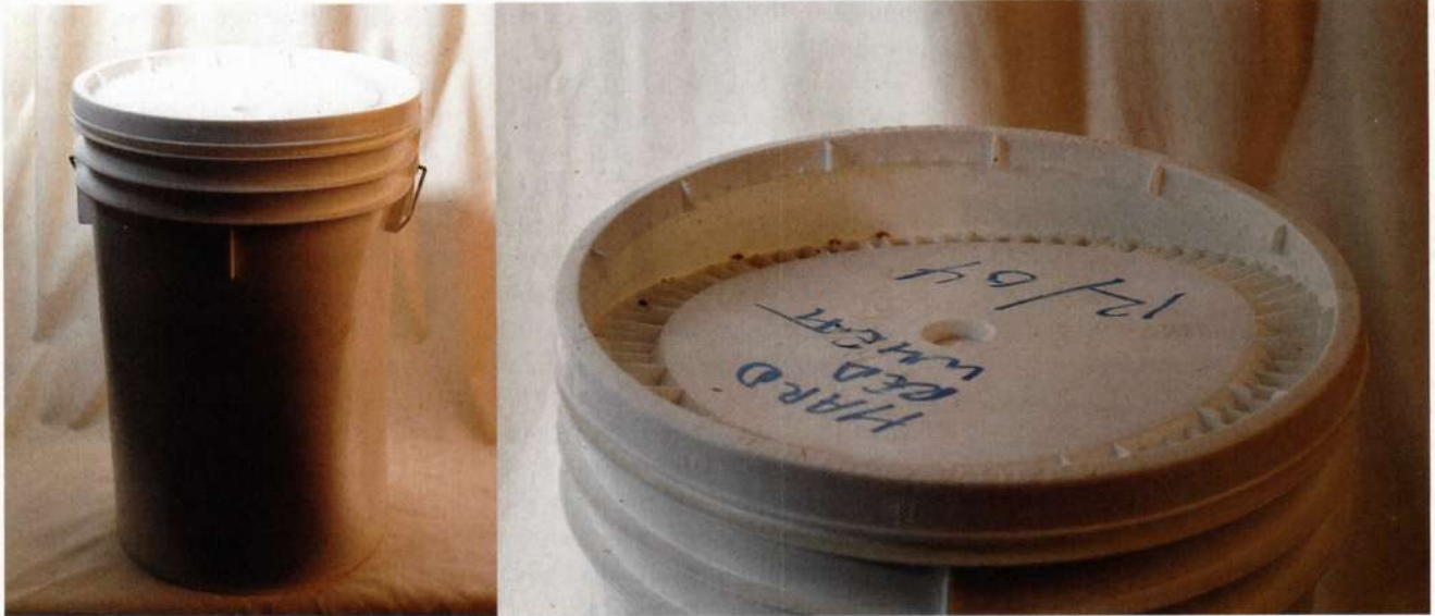
Left, A bucket of wheat under negative pressure. Right, this lid sheared off of plastic pail from negative pressure.
