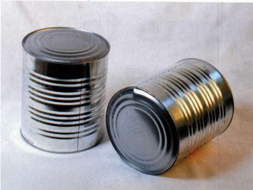
#10 cans of freeze-dried foods having premature failure (can labels intentionally removed for all photos)
